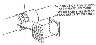
27 Apply two or more coats of sanding sealer to balsa surfaces. Sand lightly with extra fine sandpaper between coats. Repeat until pores are filled and surfaces look and feel smooth. Paint the insides of the ram tubes white, followed when dry with a coat of bright fluorescent orange paint. Cap the ends of the ram tubes with masking tape and paint all other parts of the rocket flat black.
