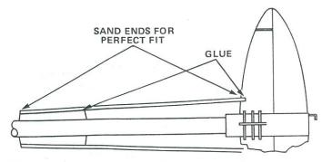
17 Test fit the conduits (1/8" diameter dowels, part L) between the sails and the conduit stand-offs. Trim the conduits to the correct length. For best result, cut the conduit pieces 1/32" to 1/16" longer than needed and then match to the sail and stand-off by sanding the ends. Glue the conduits to the sails and stand-offs. Use masking tape to hold the conduits in place while the glue dries.
