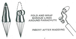
13 Fold parachute into a triangular shape. Roll 'chute tightly as shown and wrap shroud lines around it. If 'chute is too large, unroll and repack until it slides easily into rocket. A very tight fit may prevent parachute from ejecting properly.
