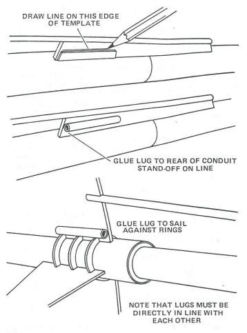
20 Cut out the launch lug location template from the pattern sheet. Mark the lug location on the conduit stand-off on the same side as the antenna platform. Glue one launch lug (part O) to the conduit stand-off on this mark. Glue the other lug to the sail--against the radiator rings and directly in line with the first lug.
