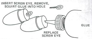
23 Insert the screw eye (part Q) into the base of the nose cone (part R). Remove screw eye and squirt a small amount of glue into the hole. Re-insert the screw eye.
