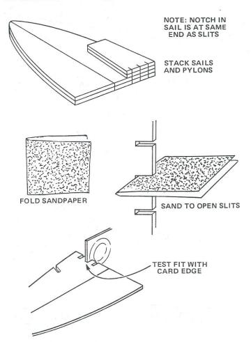
11 The sails and the engine pylons each have three slits die-cut in their root edges. Stack these four parts so the slits match. Fold a piece of extra fine sandpaper and use it to open the slits until the die-cut card material (part K) fits snugly in the slits.
