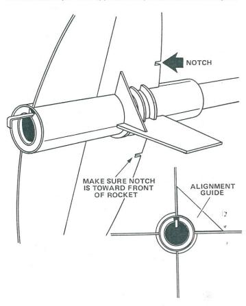
Apply a line of glue to the root edge of a sail and rub it into the wood. Allow glue to set. Apply another line of glue and position the sail on the body with the radiator rings in the slits. Use the alignment guide from the die-cut card (part K) to make sure the sail projects straight out from the body. Install the remaining sail and the engine pylons this way. When the sails and pylons are in position, apply glue to the joints between balsa parts and the body. Let the assembly dry.
