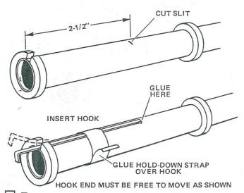
Qut a 1/8" slit in the body, directly in line with the gap in the split adapter ring, 2-1/2" from the end of the body. Cut out the hold-down strap from the pattern sheet (part G). Insert one end of the engine hook (part H) into the slit and lay the hook along the body so the other end passes through the gap in the split ring. Smear glue over one side of the hold-down strap and wrap it around the body, centered over the hook. Apply a drop of glue over the forward end of the engine hook.
