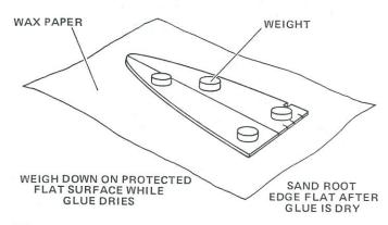
Quart J). The best method is to first sand both sides of each sheet smooth, then free the parts, where necessary, with a sharp knife. Glue the sails together as shown, making sure you match one notched and one unnotched half. Lay the sail assemblies flat on a piece of waxed paper and weight down to hold in position while the glue dries.
