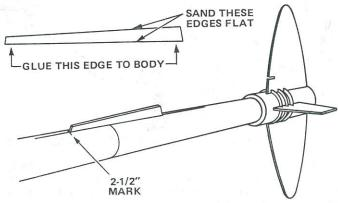
15 Glue the conduit stand-offs to the main body on the lines drawn in step 14, directly ahead of the sails. The front edge of each conduit stand-off should be on the 2-1/2" mark.
