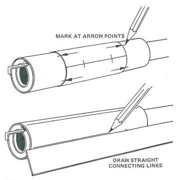
10 Cut out the reactor body marking guide from the pattern sheet. Wrap it around the reactor body and mark at each arrow point as shown. Use a ruler to draw a straight connecting line between each matching pair of marks.
