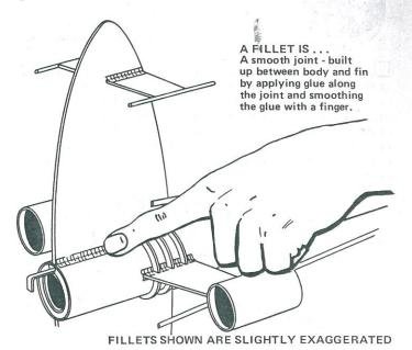
**24** Apply a glue fillet to each joint where a sheet balsa part connects to another part. Holding the rocket horizontally, apply a line of glue to the joint and smooth it out with your finger. Support the rocket horizontally while the glue dries.
