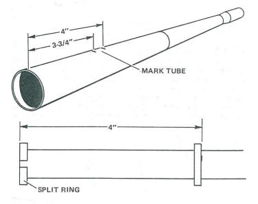
6 Mark the rear end of the body assembly 3-3/4" and 4" from the end. Apply a line of glue around the tube at the 3-3/4" mark and slide the remaining adapter ring (part D) onto the tube until the front end of the ring is even with the 4" mark. Wipe away any excess glue immediately. Glue the split adapter ring (part F) to the tube so it is even with the rear end.
