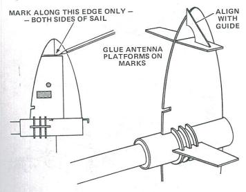
16 Cut out the antenna platform location template from the pattern sheet. Mark both sides of one sail on the outer edge of the template. Glue the antenna platform pieces to the sail on the location lines. Use the alignment guide to be sure the antenna platforms project straight out from the sail.
