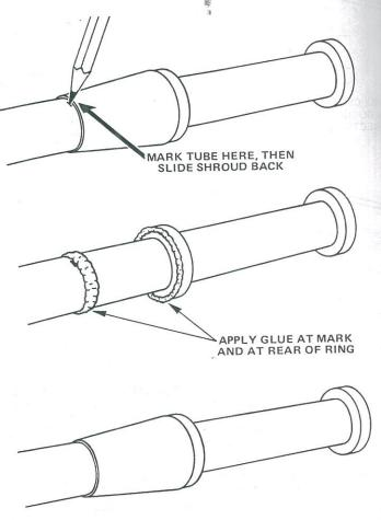
4 Slide the shroud onto the body and up against the first ring as shown. Mark the body where the end of the shroud touches it. Slide the shroud back and apply a line of glue around the body at the mark and around the ring where the shroud will touch. Slide the shroud back into position.
