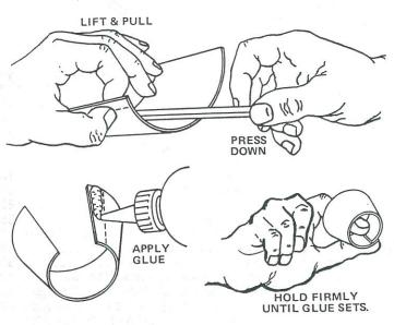
2 Pre-form the shroud (part C) by pulling it under a knife handle or pencil as shown. Pull the shroud under the handle or pencil and up at the same time. Do this several times until the cone can be formed easily. Apply glue to the tab on the cone and press into position exactly as shown. Hold it in place until the glue sets.
