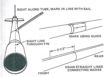
14 Sight along the main body from the front and mark it at the middle, straight forward from a sail. Cut out the main body marking guide from the pattern sheet and wrap it around the body, matching one arrow point to the mark. Mark at the other three arrows. Use a ruler to draw a straight line connecting matching marks. Extend lines at least 3" on each side of the joint in the main body. Mark each line 2-1/2" ahead of the joint.
