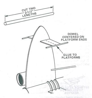
19 Cut two 2-1/2" long antennas from the 1/12" dia. dowel (part N). Glue the antennas to the antenna platforms. The antennas should be perfectly centered on the ends of the platforms.
