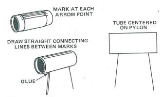
■ 18 Cut out the ram tube marking guide from the pattern sheet. Wrap it around a ram tube (part M) and mark at each arrow point. Repeat with the other ram tube. Glue the ram tubes to the engine pylons using the pylon position marks. Check alignment of each with the die-cut guide.
