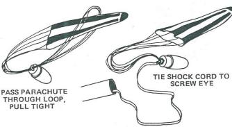
26 Cut out the parachute (part S) on its edge lines. Cut three 36" lengths of shroud line (part T). Attach line ends to top of parachute with tape discs (part U) as shown. Pass shroud line loops through screw eye. Pass parachute through loop ends and draw lines tight against screw eye. Set knot with a drop of glue. Tie free end of shock cord to screw eye.
