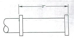
Mark the body assembly 2" and 1-3/4" from one end. (This will be the front of the model.) Apply a line of glue around the body at the 1-3/4" mark and slide an adapter ring (part D) onto the tube, over the glue, until it just touches the 2" mark. Glue a second ring on this end of the body so the front edge of the ring and the front edge of the body are even.
