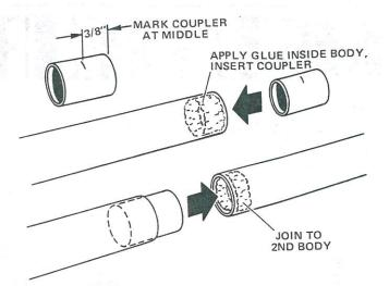
Assemble the main body. Mark the tube coupler (part A) at its middle. Smear glue around the inside of one end of an 18" body tube (part B). Insert the coupler into the glued body end so half of the coupler is in the tube. Let the glue set, then smear glue inside one end of the other 18" tube and slide glued end onto the coupler to join the tubes. Lay the assembly on a flat table top and roll gently to make sure the tubes are straight.
